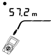
Figure 6.15 Open on Coaxial Cabling
