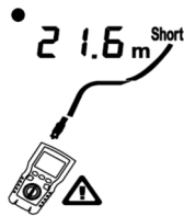
Figure 6.16 Short on Coaxial Cabling
