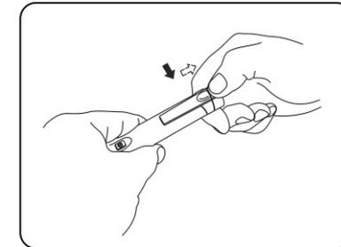
(2). Please take out the upper cover of test pencil according to the direction as shown in the picture, replace the battery. (see the following picture)
